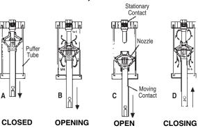
**A.** The stationary contact and piston assembly (containing the moving contact and nozzle) are housed in clear cylindrical tubes. These are mounted in a modular three-phase assembly which is independent of the switch tank. The stationary contacts are supported independent of the cable entrance bushings, eliminating possible
