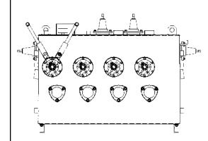
RAM44 with top mounted bushings and operators.
