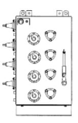
Vertical mount VRAM44 with side mounted bushings and front operators.
