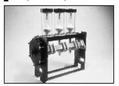
▲ Three phase linear puffer mechanism.
