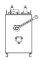
RAM21 with top mounted bushings and front operator.
