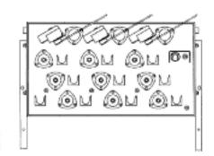
RAM 33 with front mounted bushings and operators.
