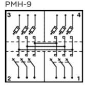
Figure 3 – Air insulated Switchgear 9 Configuration
