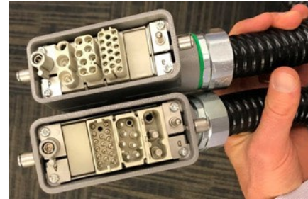
Main Control Cable Connectors with Protective Cable Armor
