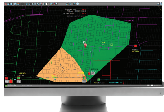
FLISR (Fault Locations, Isolation and Service Restoration) shown on a monitoring computer
