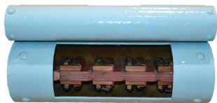
Close up of the severed main conductor and melted current limiting element of a 3000A (double bus) CLiP after interruption
